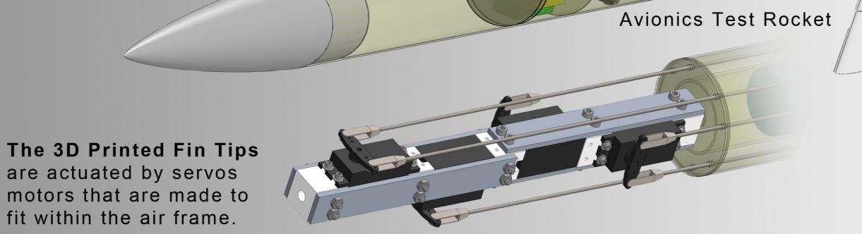
Fin section will be competely modular to allow for different fin configurations.
