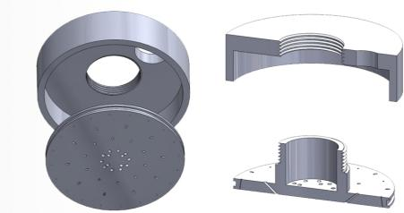
The Injector Plate will channel the correct ratio of LOX and Kerosene into the chamber.
